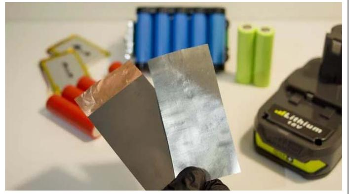
For years, mass-produced lithium-ion batteries have relied on graphite and copper for their anodes, the component that stores the energy as the battery charges. And for years, researchers have sought out alternative materials that could overcome the limitations of those materials, which include a high cost of production and limited storage capacity (silicon, for example, **could store 10 times** as much energy, although it poses another set of problems).
